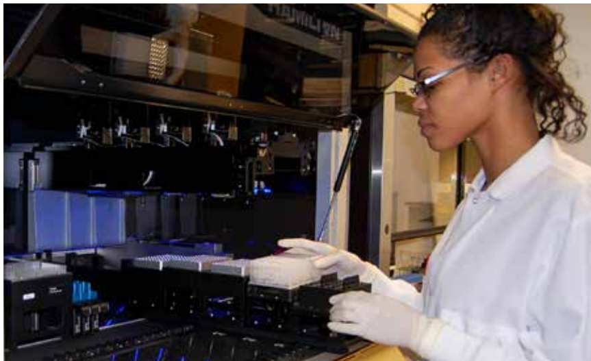
An examiner at the Kansas City (Mo.) Police Department Crime Laboratory loads a DNA plate onto a liquid handler robot. Photo courtesy Jennifer Howard, Kansas City Police Department Crime Laboratory
