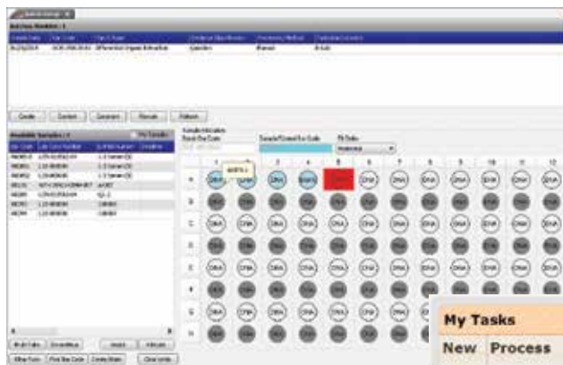
▲ The batch setup module in a sample tracking and control program allows the user to allocate samples to batches. Image courtesy STACS DNA
